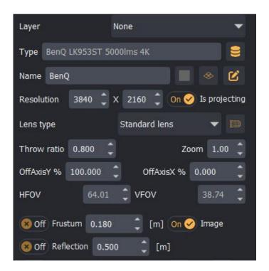
Now we will continue and we will use Designer PRO to assist us to position and orient the projectors to the designed position and orientation.
